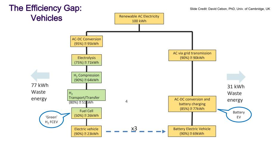
3x more renewable electricity to power a hydrogen FCEV than a Battery EV: 3x cost!
