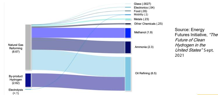
Figure 1: Current Hydrogen Supply and Demand Balance in the United States (Mt)<sup>22,23</sup>
