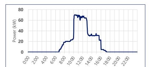
**10am Floodgates**: Charging maximized to transformer limits during 10am-2pm to optimize for incentives for consuming surplus solar energy
