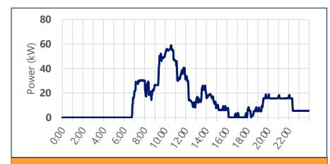
**Max Delivery:** Load management delivered as much power as desired within the 75kW constraint
