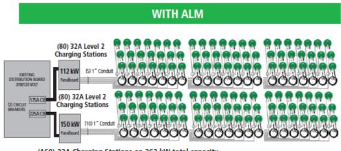
(160) 32A Charging Stations on 262 kW total capacity using UL916 Adaptive Load Management
