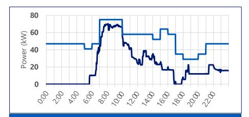
**LCFS Curve Following**: Charging optimized under LCFS Time-of-Use Value curve
