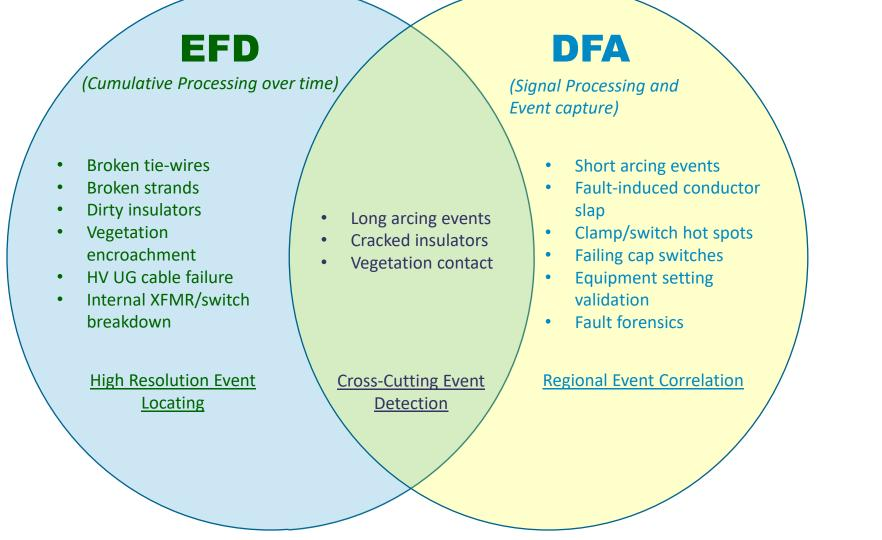
Types of events detected are driven largely by cumulative detection (employed by RF Sensors) vs. continuous monitoring of waveforms and signal processing to detect single/infrequent period event (employed by DFA)
